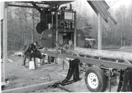
The school purchased a newer, safer, portable sawmill to use in sawing lumber for pallets.
